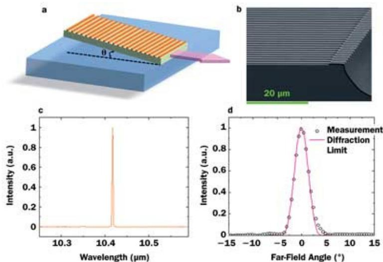
Manijeh Razeghi, the Walter P. Murphy Professor of Electrical Engineering and Computer Science at Northwestern University's McCormick School of Engineering and Applied Sciences, and colleagues developed the resonator using a new type of distributed feedback mechanism called B-DFB, a simple diffractive feedback in an angled laser cavity.
